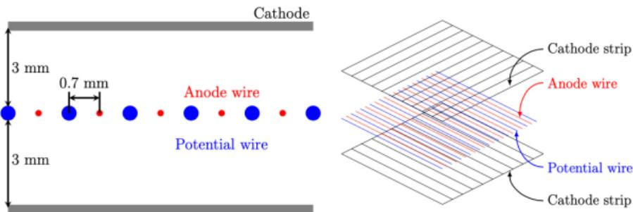
fig 1: Schematic of HV-switching MWPC
